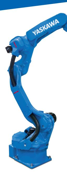
The MOTOMAN GP12 is a fast and precise 6-axis industrial robot with a payload capacity of up to 12 kg. With a reach of 1440 mm and a high repeatability of  $\pm$  0.02 mm, it is ideally suited to assembly tasks, but also universal handling tasks, CNC machine tool tending or packaging. Its streamlined modern industrial design minimizes the space requirements at the installation site.
