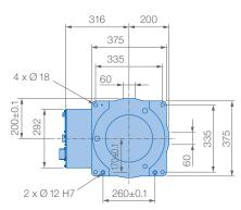
Mounting options: Floor, ceiling, wall, tilt\* Protection class: Main axes (S, L, U) IP54, wrist IP67
