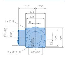
Mounting options: Floor, ceiling, wall, tilt\* Protection class: Main axes (S, L, U) IP54 (option IP65), wrist IP67
