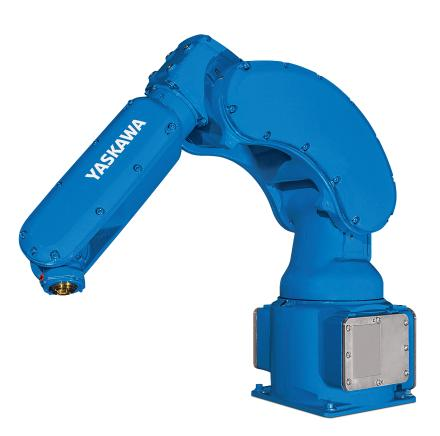
The compact MOTOMAN MPX1150 robot was developed especially for painting of small work pieces. It provides a payload of 5 kg for mounting multiple guns and small bells. Its high density layout saves space by reducing the size of the painting booth. The S/L axis is designed with no offset to enable installation of the manipulator closer to a work piece. The robot can be mounted on the floor, wall or ceiling and has three selectable access points for power cables.
