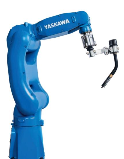
The MOTOMAN AR700 is a compact high-speed 6-axis robot which provides accurate performance to achieve optimal results in extremely difficult conditions and especially for the high demands of arc welding applications.
